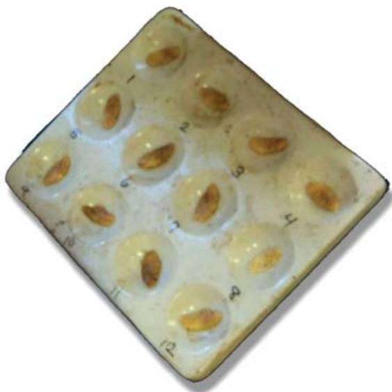
Figure 3.51. Baked otoliths in tray.
