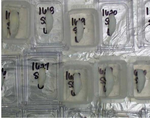
Figure 3.6. Embedding molds labeled with identification information.
